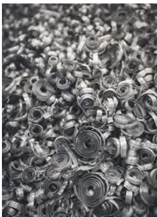
The milling process can produce up to 300 kilograms of chips per hour.
