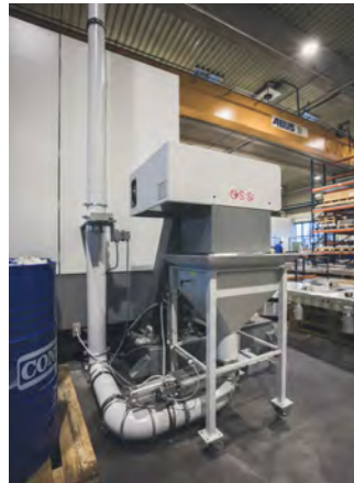
Automatic extraction and swarf handling on CNC milling machines: That's how chips become valuable raw material again during operation.
