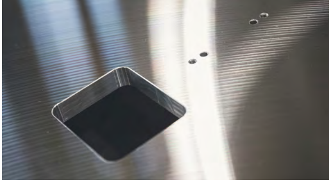
Milling is carried out with micrometre precision. One component can take up to 50 hours to machine.
